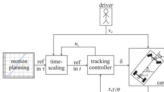
**Fig. 4.** Scheme of the tracking controller with time-scaling
