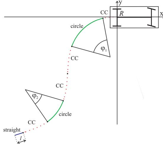
**Fig. 3.** Reference path for parking in a lane
