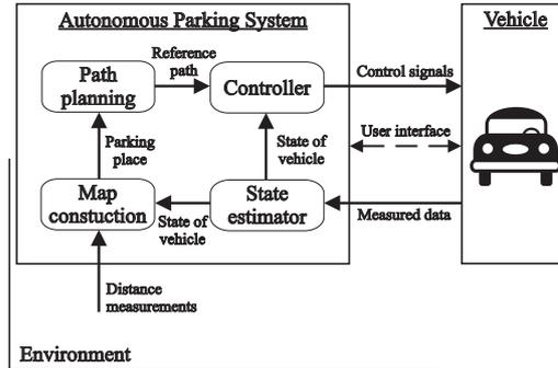
**Fig. 1.** Components of the Automatic Parking Assist System
